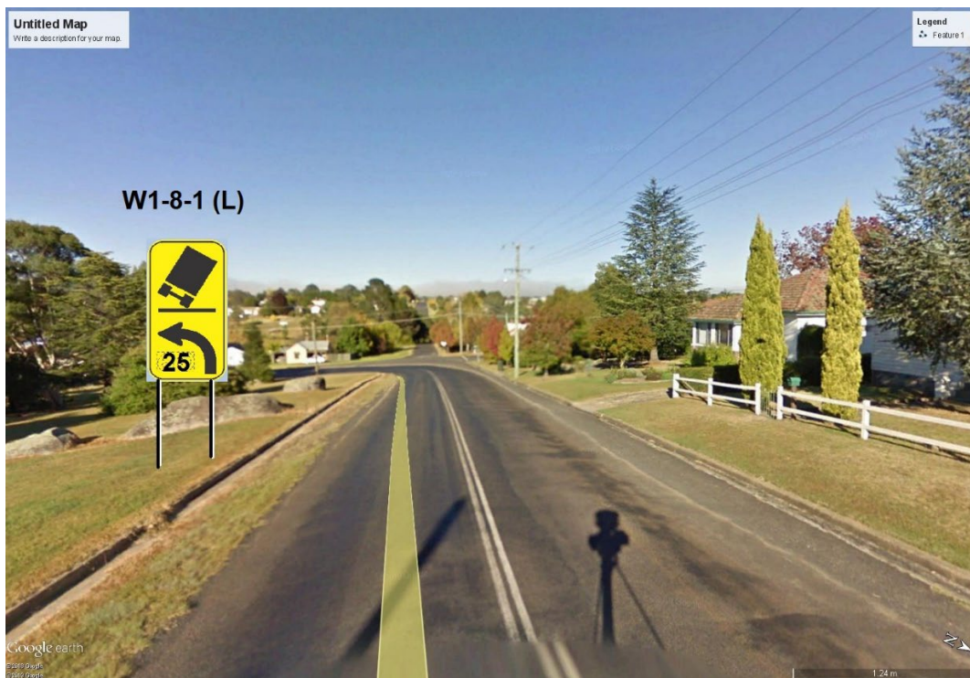
Figure 2 - Mark-up provided by TfNSW (now installed)
