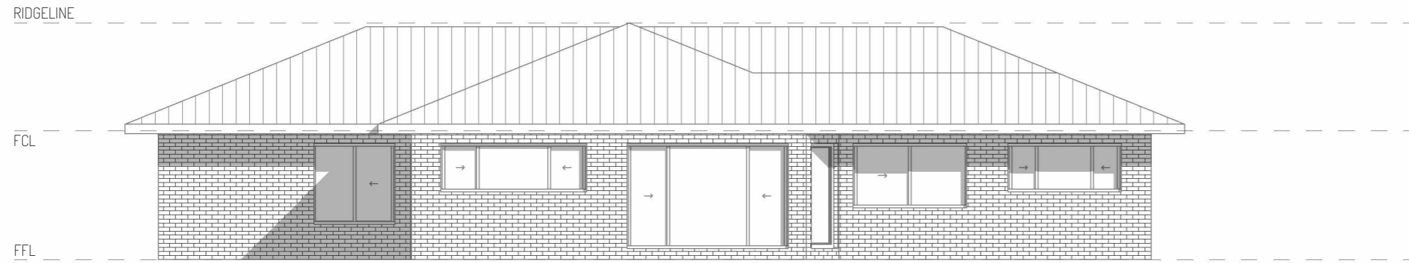
1 EXISTING ELEVATION, NORTH 1:100
