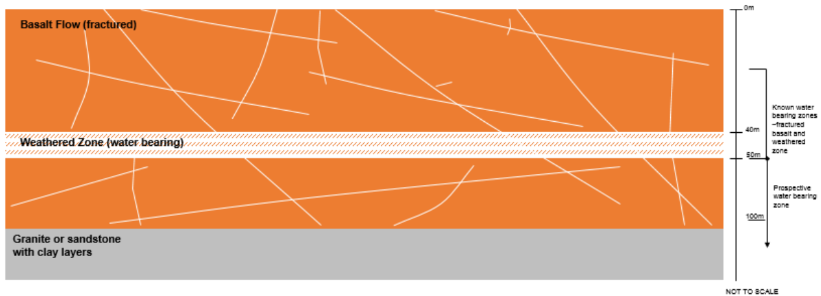
Uralla Groundwater Project – Conceptual Geological Strata and Water Bearing Zones
